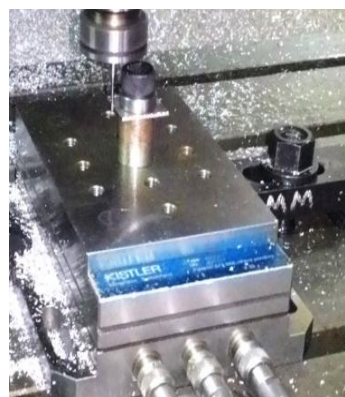
Fig.9 Measurement of cutting forces by a dynamometer
