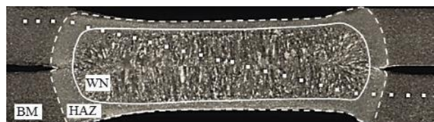
Fig. 5 Typical cross-section of weld under the condition of fourth test and corresponding of Vickers hardness across the weld
