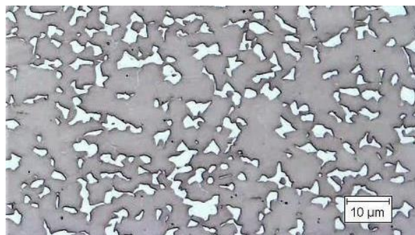
Fig. 3 Microstructure of dual phase steel
