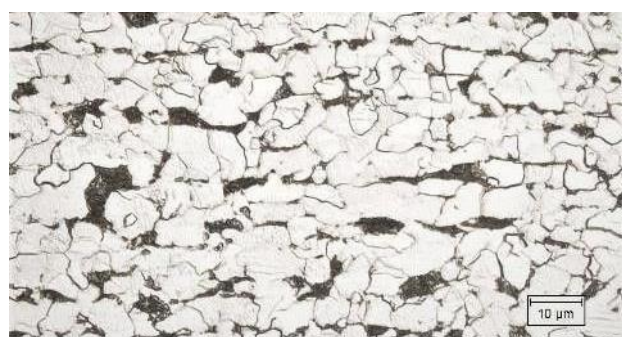
Fig. 2 Microstructure of ST52-3
