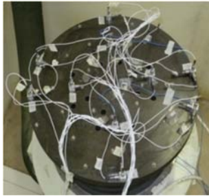
Fig. 5 Vibration sensors arrangement on head expander
