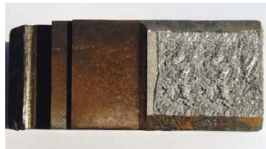
Fig. 9 Fatigue and fracture surface of CT specimen
