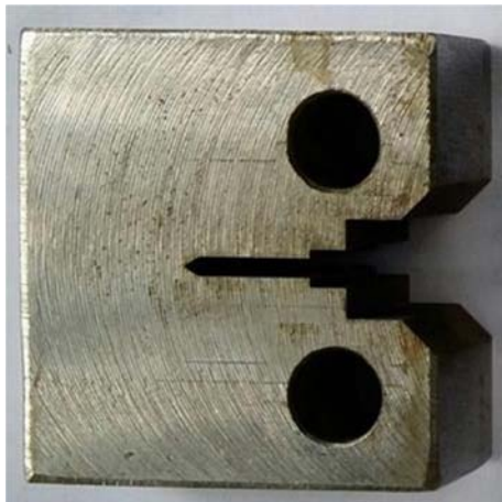
Fig. 5 Photograph of a machined CT specimen
