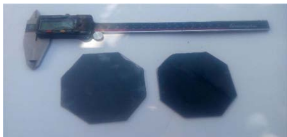
Fig. 12 Initial blank for experiments with two drawing ratio
