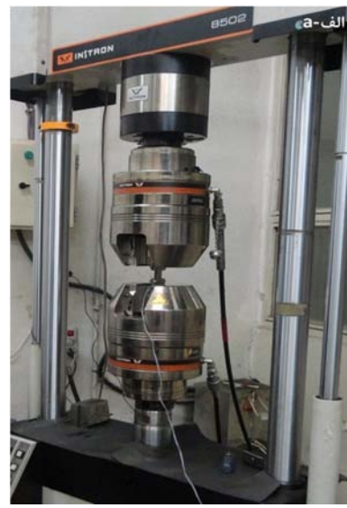
Fig. 4 a- INSTRON 8502 servo hydraulic machine b-schematic of sample position between the guide and the attached strain gauge
