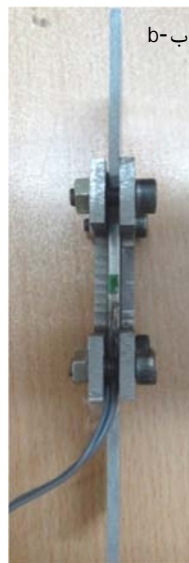
Fig. 4 a- INSTRON 8502 servo hydraulic machine b-schematic of sample position between the guide and the attached strain gauge
