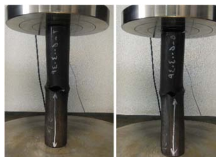
Fig. 5 figure of (5-2-C 125) and (5-5-L 125), after buckling
