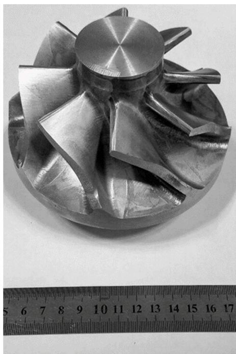
Fig. 20 machined impeller by 3+2-axis machining method
