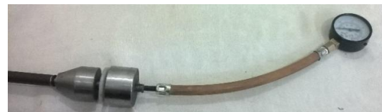
Fig. 9 Pressure gauge connection to the main axle
