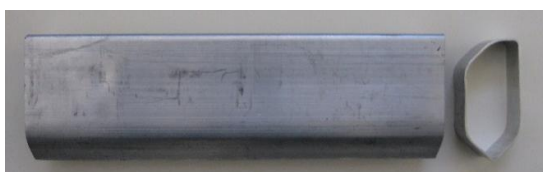
Fig. 21 The test result for tube filled with water at pressure equal to 8 bars using the three-piece die
