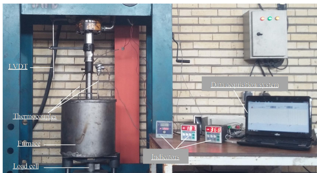
Fig. 1 Components of the data acquisition system and their placement
