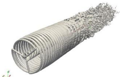
Fig. 17 Vortex isosurface contours and wakes structure
