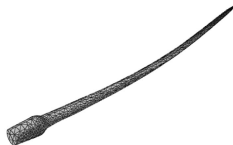
Fig. 11 The first bending mode of turbine blade vibration in ABAQUS software
