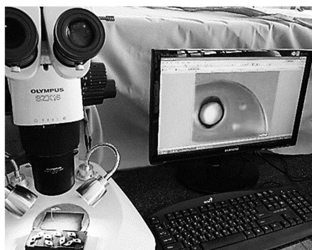
Fig. 3 Measuring setup of tool wear using SZX16 optical microscope
