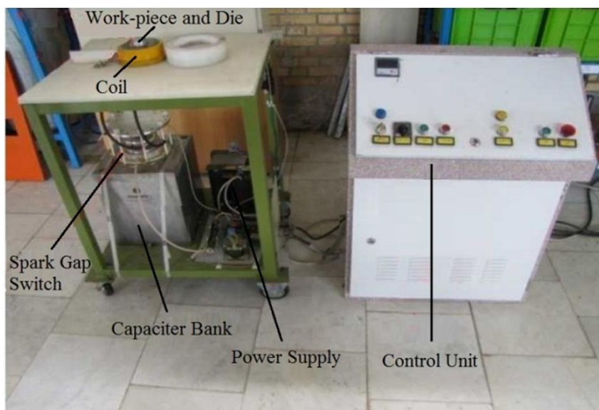
Fig. 6 Electromagnetic Forming Equipment
