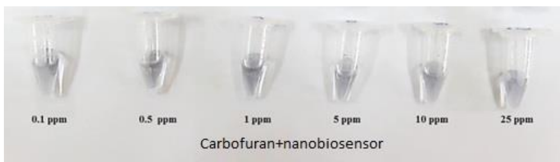
Figure 8 Specific accumulation of nanobiosensors in the presence of different concentrations of carbofuran.
