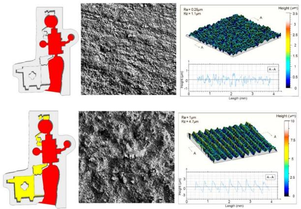
Fig. 12. Architectural Plan of Maraghe Tomb. According to The Results of Laser Scan Date Towards Curved Surfaces of the Structure; The Older Part (Red) Whit Its Polished Surface Is in Contrary with The Additional Parts (Yellow) As an Evidence That Two Distinguishable Surface Reveals Two Probable Constructions Phases.
