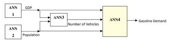
Fig 2 Structure of Designed Hierarchical ANN
