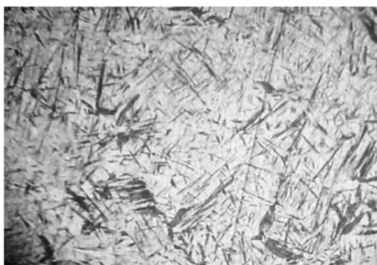
Fig. 4 Steel (1.1191) with Microstructure of Martensite
