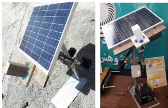
Fig. 10 Fabricated dual-axis sun-tracker under test conditions.
