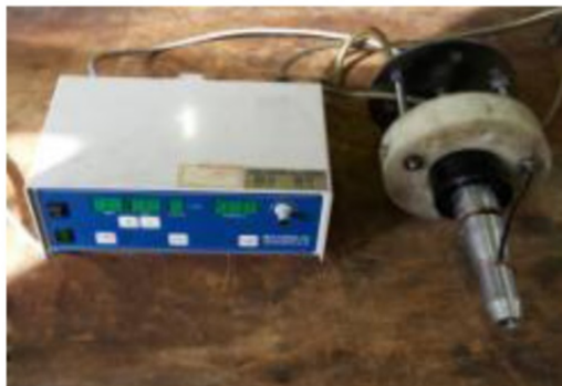
Fig.1 The ultrasonic vibration generator used for machining
