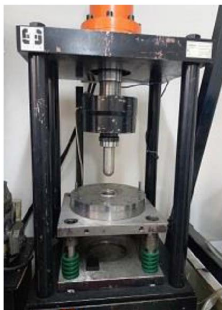
Fig. 6 The hydraulic press used to perform the Nakazima test
