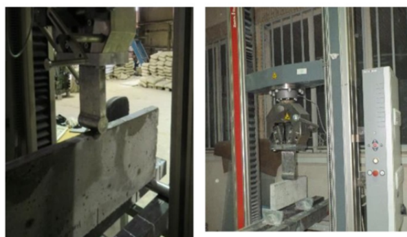
Fig. 2 Test setup configuration for three-point bending tests
