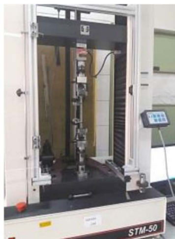
Fig.2 Santam tensile test machine (5Ton)
