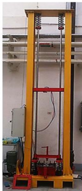
Fig. 3 Low velocity impact test machine (Drop Weight)
