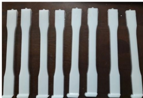
Fig. 1 fabricated specimen by injection molding
