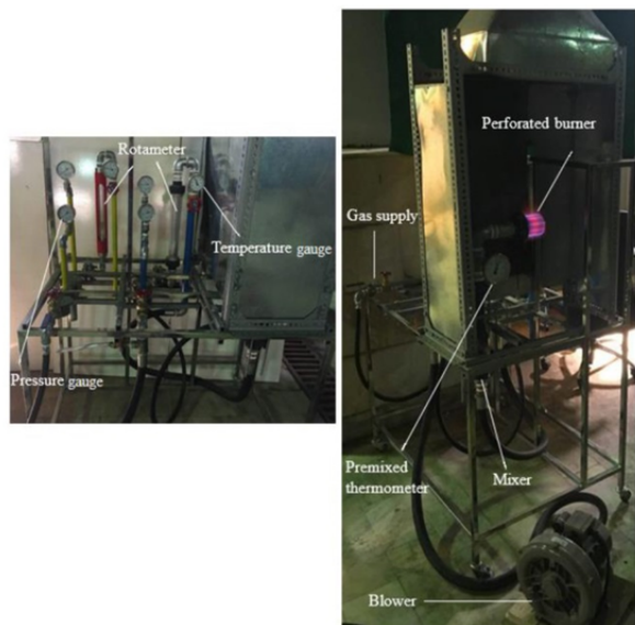
Fig.5 The designed and fabricated test rig of the premixed perforated burner
