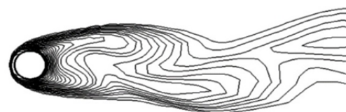
Fig. 21 Instantaneous temperature contour at Re = 150
