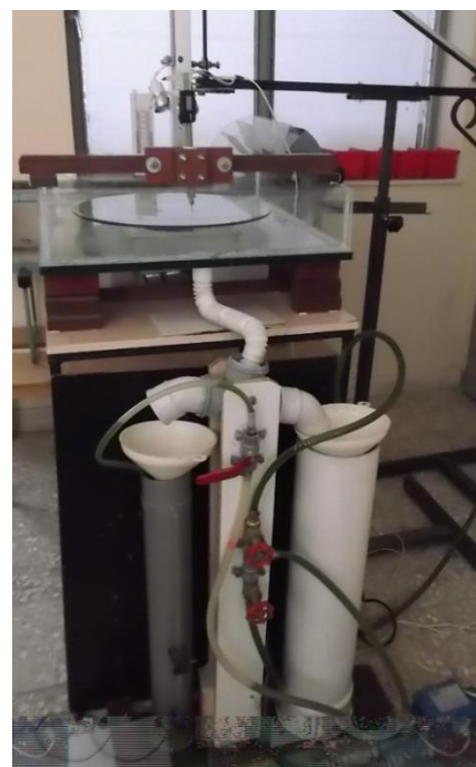
Fig. 2 The apparatus of the hydraulic jump in used for this work
