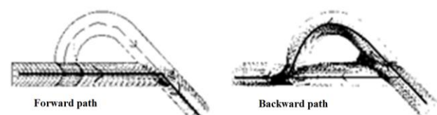
Fig. 1 The effect of difference between conjunction angles on the creation of diodicity property [1]
