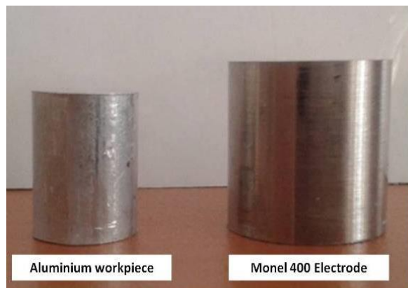
Fig. 1 Monel Electrode and workpiece
