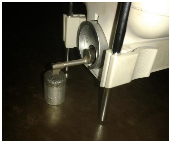
Fig. 3 Surface roughness Measurement after discharge operations
