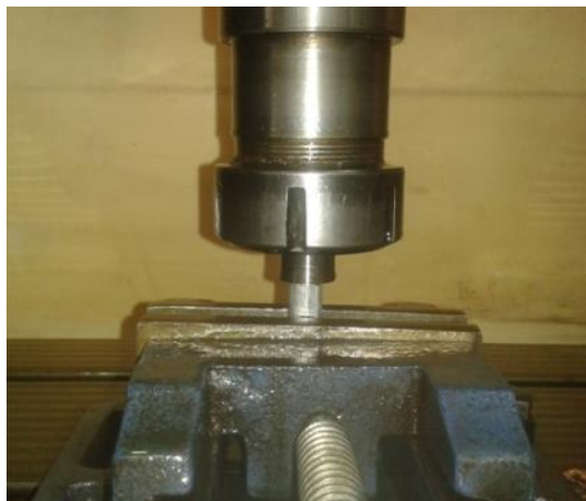
Fig. 2 Setting the electrode to electrical discharge process
