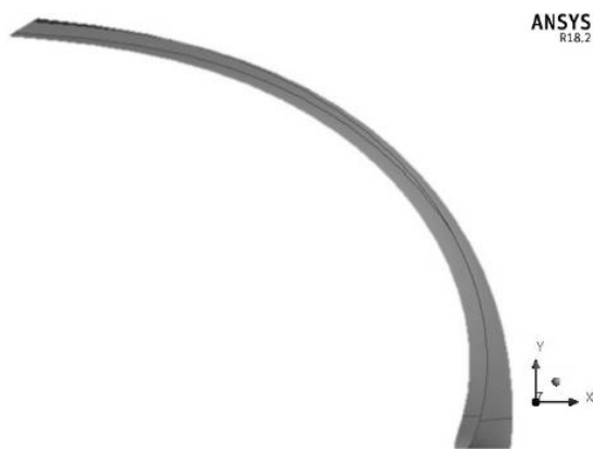
Fig. 15 The original blade of centrifugal pump
