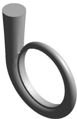
Fig. 2 Designed volute with CFTurbo software
