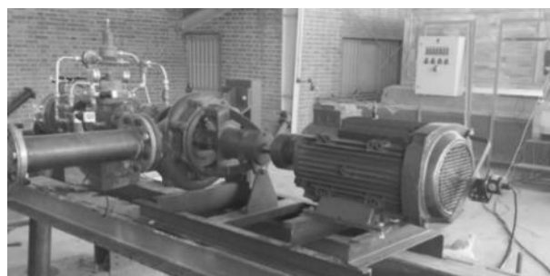
Fig. 10 Reverse pump in test circuit
