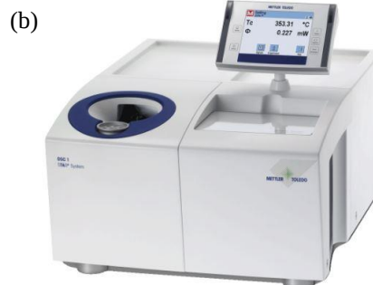
Fig. 4 a- DSC test results and adopting phase transformation temperatures from the Heat Flow-Temperature diagram, b- DSC test setup
