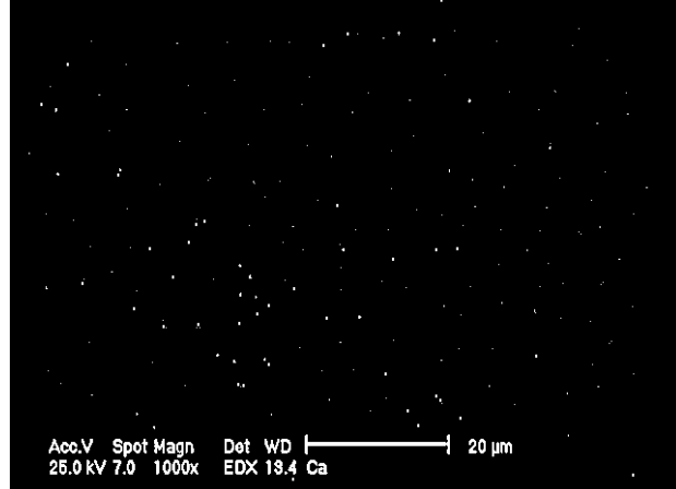
Fig.9 SEM image of coated scaffold &amp; calcium map
