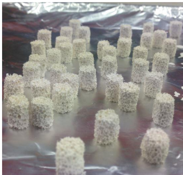
Fig.2 Stain foam to ceramic solution
