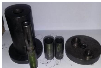
Fig. 2 Schematic of used PTCAP die and its components
