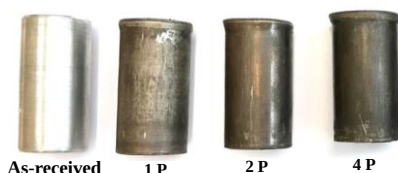
Fig. 4 Pictures of unprocessed and one, two and four-pass PTCAP processed samples
