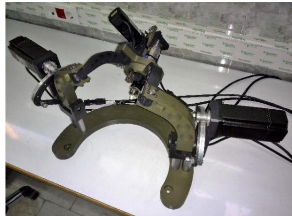
Fig. 14 Final detail design and prototype of the 3-DoF mechanism
