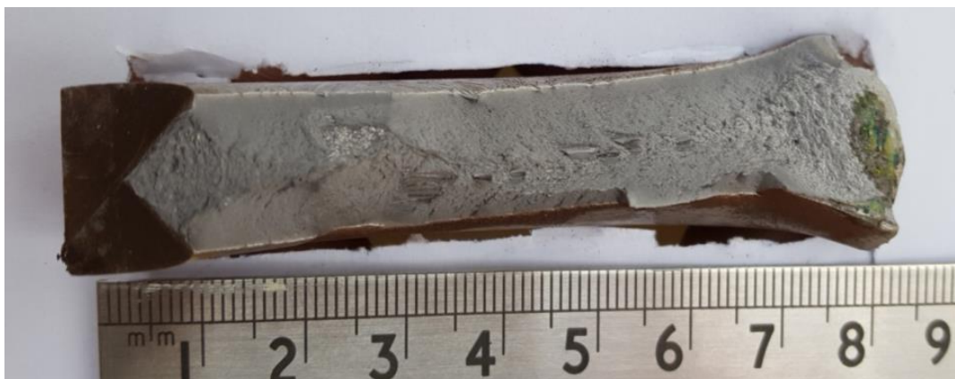
Fig. 15 Fracture surface of right part of DWTT specimen with crack growth direction from left to right
