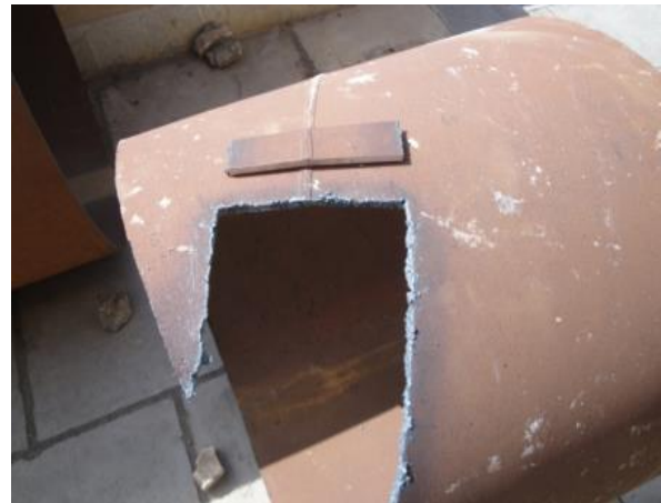
Fig. 3 Specimen machined from an actual gas pipe with spiral seam weld
