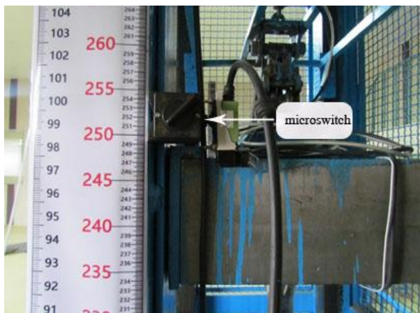
Fig. 6 Microswitch used on DWTT machine for exact adjustment of hammer height
