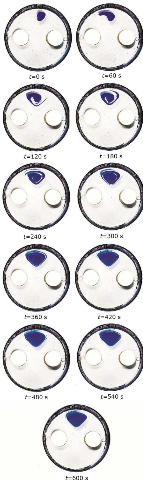
Fig 4 Dye mixing in the mixer with constant speed of rotors
