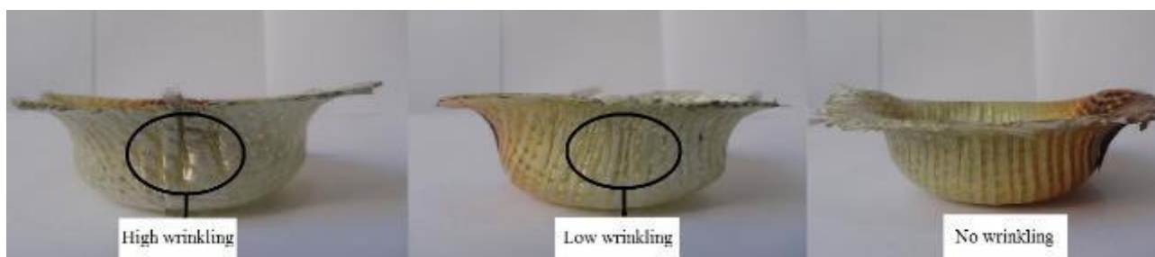
Fig. 12 Result of experimental tests for wrinkling of PVC/fiber glass composite laminates
