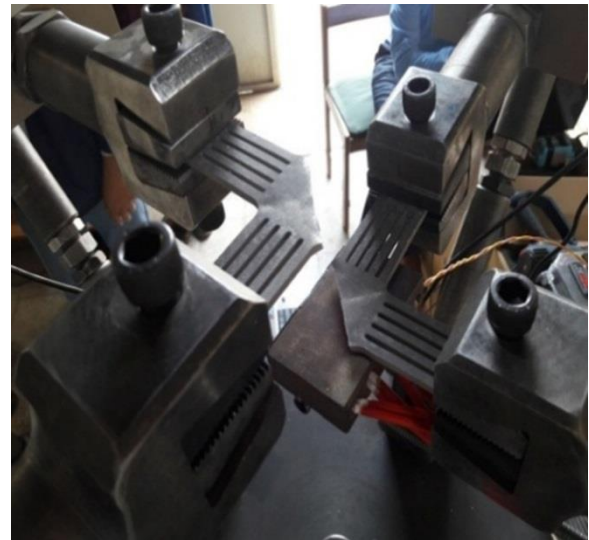
Fig. 8 The cruciform specimen fracture from Al. alloy 5083
