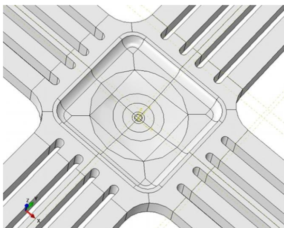
Fig. 10 The cruciform specimen partition in ABAQUS software; the x axis is rolling direction and y axis is transverse direction
