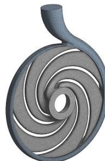
Fig. 3 Computational mesh for impeller and volute
