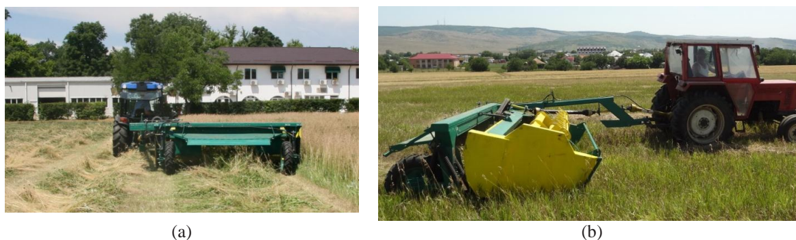
Figure 3. The trailed vinderover on experimental plots: (a) INMA Bucharest field, (b) SCDP Vaslui field.
