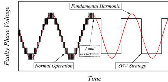
Figure 4. Square wave voltage post-fault operation strategy
