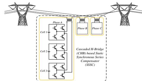
Figure 1. Cascaded H-bridge multilevel converter as an SSSC
