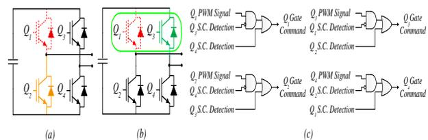
Figure 2. Structural reconfiguration strategy for a faulty HB cell (a) The short-switch fault occurs in  $Q_1$  and the gate command for  $Q_2$  becomes active. (b) The damaged HB cell should be bypassed by  $Q_1$  and  $Q_3$ . (c) The proposed protection scheme for a faulty HB cell
